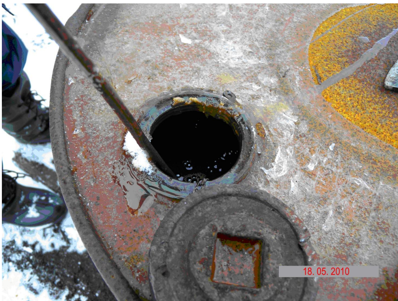
Figure 22. Testing Motor Oil Drums for PCB
