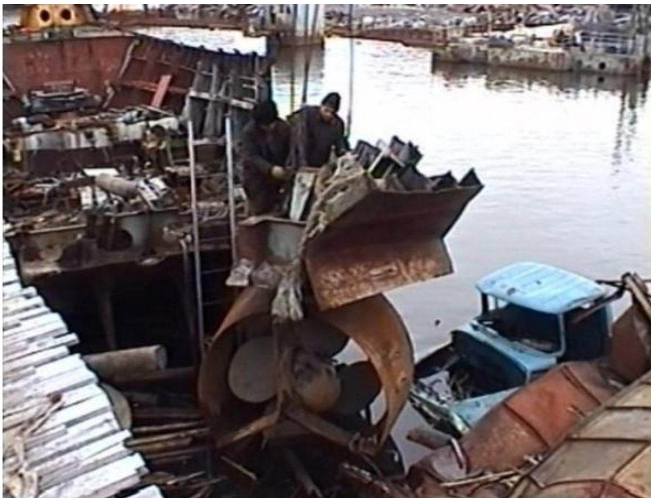
Figure 26. Cutting and Utilization of Ship Lifted from Sea Floor
